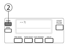
You can gradually decrease the washing water temperature between the maximum temperature and cold washing (--) by pressing washing water temperature adjustment button.
